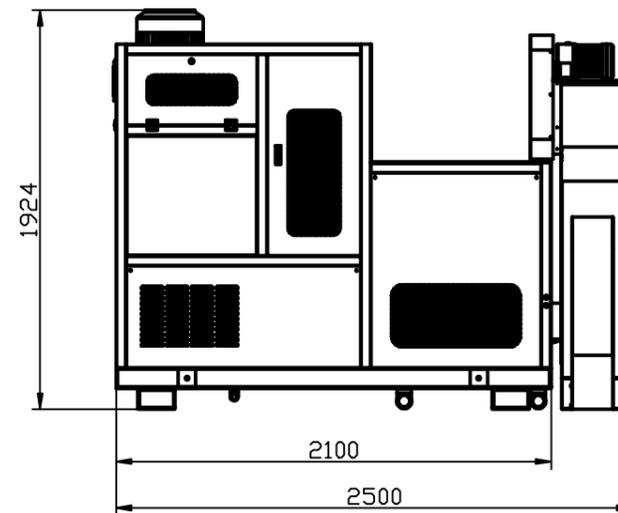
Extrusion force : 1000kN
