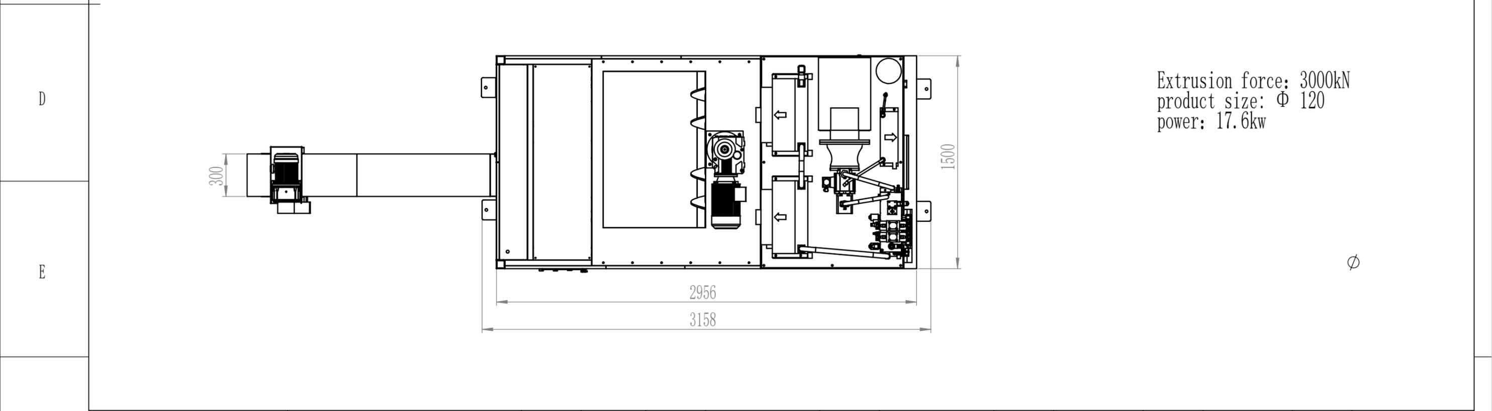
Extrusion force: 3000kN
